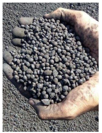
✤ It contains whopping 74,000 PPM of sulphur content which is released into atmosphere as emissions which is much higher than vehicular emissions.
