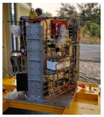
✤ ISRO has successfully tested a 100 W class Polymer Electrolyte Membrane Fuel Cell based Power System (FCPS) in its orbital platform, POEM3.
