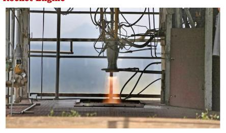
❖ ISRO successfully conducted hot testing of liquid rocket engine manufactured through 3D printing technology.
