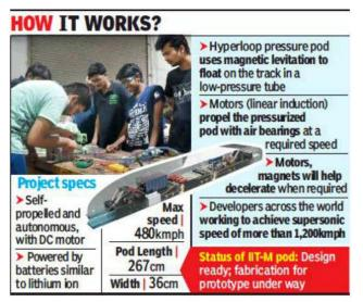
It is an indigenous design and development for building the first-ever selfpropelled, completely autonomous Hyperloop Pod in India.
