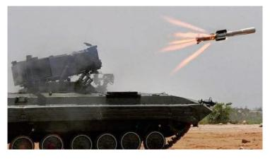
❖ NAMIS system includes - a 3rd generation Anti-Tank Guided Missile, the NAG and Missile Carrier Vehicle (NAMICA).
